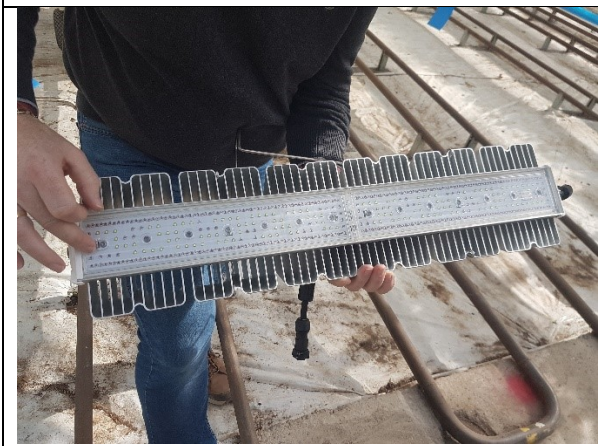
Figure 3 One of the lights. These are efficient LEDs. But they still consume 2.8 megawatts in total!
